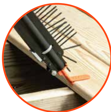
Use the Edge nose piece with CAMO Collated Edge Screws (p. 12)
